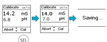
\*Stabilize: When drawing solution into the meter, a stable reading is defined as maintaining a constant value or value is switching between 2 neighboring numbers (i.e. 14.0-14.1)
